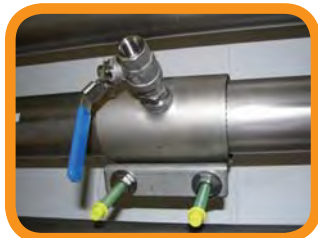
Spot drilling collar
