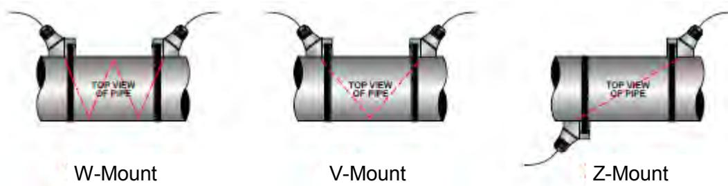
Illustration 1: Transit-time sensor mounting configurations
